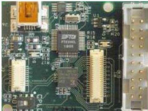
Figure 2.1) Intel Mote 2 Debug Board
