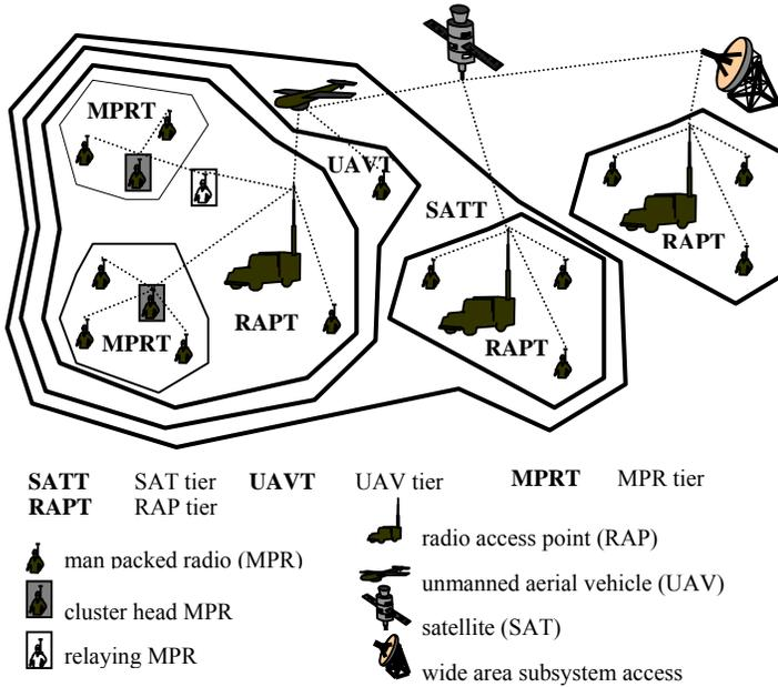
Figure 2. Architectural elements of the mobile subsystem [17].
