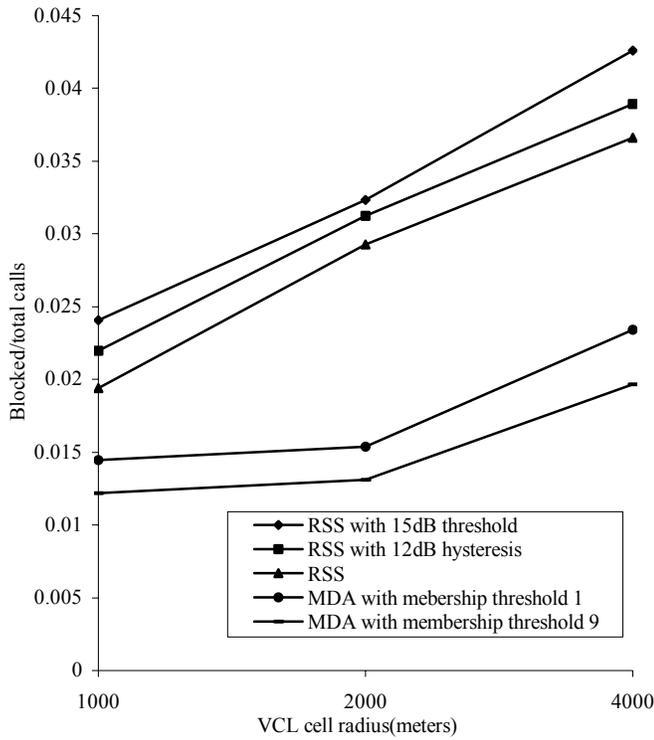
Figure 13. Comparison of handoff decision algorithms for the second scenario, in terms of blocked calls due to lack of network resources for the multiplication factor 2.
