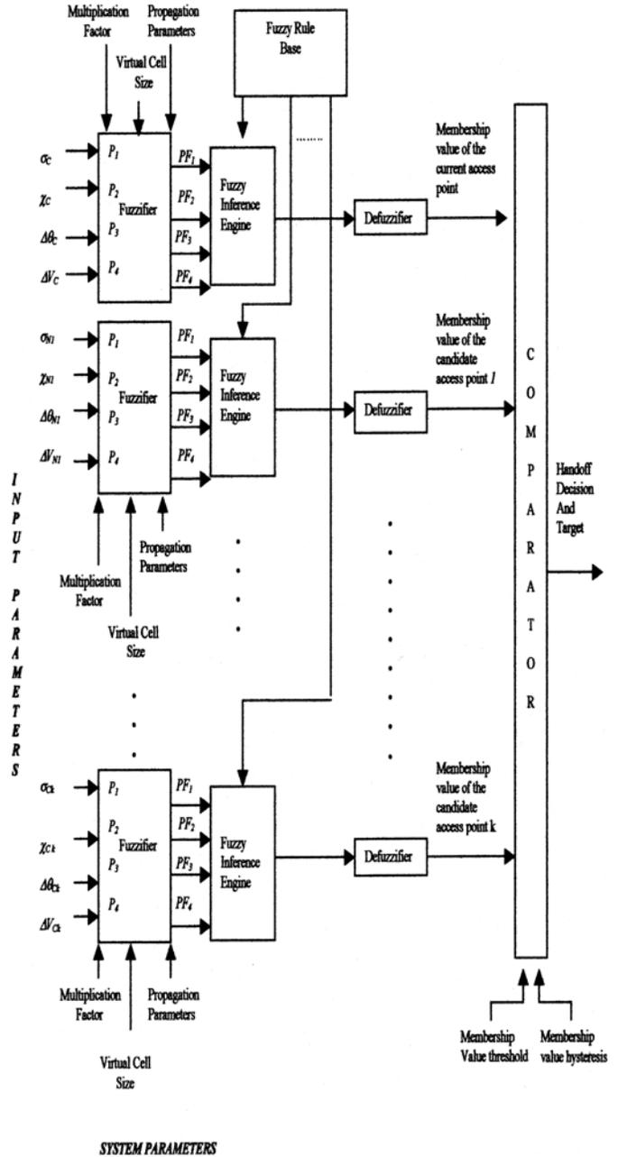
Figure 4. Block diagram of the handoff decision system.
