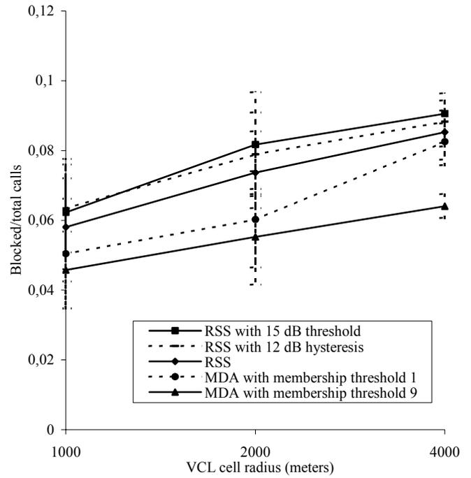
Figure 8. Comparison of handoff decision algorithms in terms of blocked calls due to lack of network resources for the multiplication factor 1.
