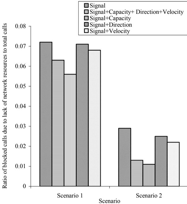
Figure 16. Partial effect of the handoff decision components on the ratio of blocked calls due to lack of network resources to total calls.
