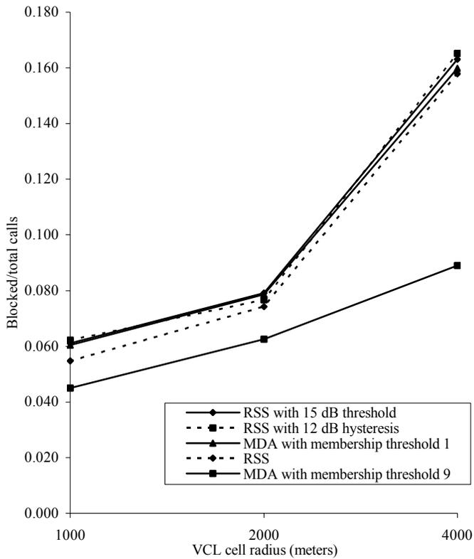
Figure 10. Comparison of handoff decision algorithms in terms of blocked calls due to lack of network resources for the multiplication factor 2.
