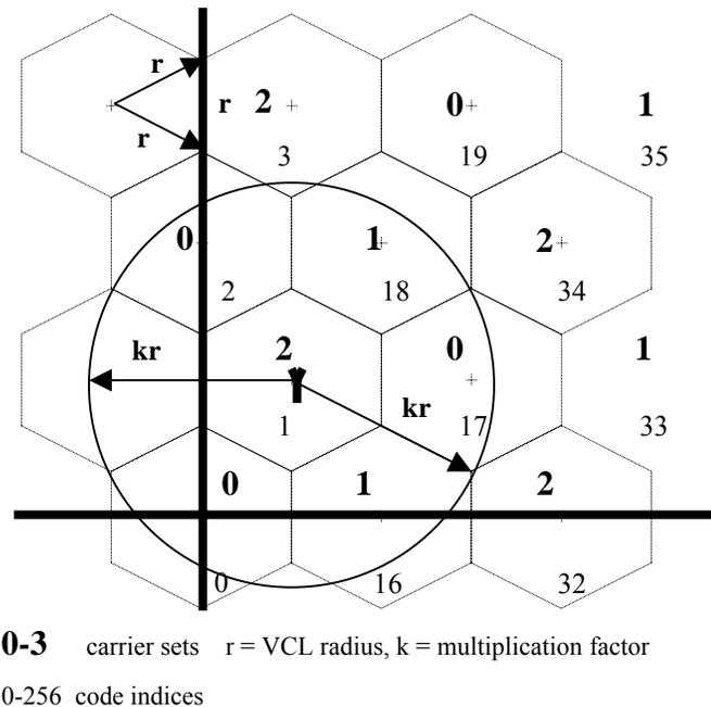
Figure 3. Virtual cell layout [17].
