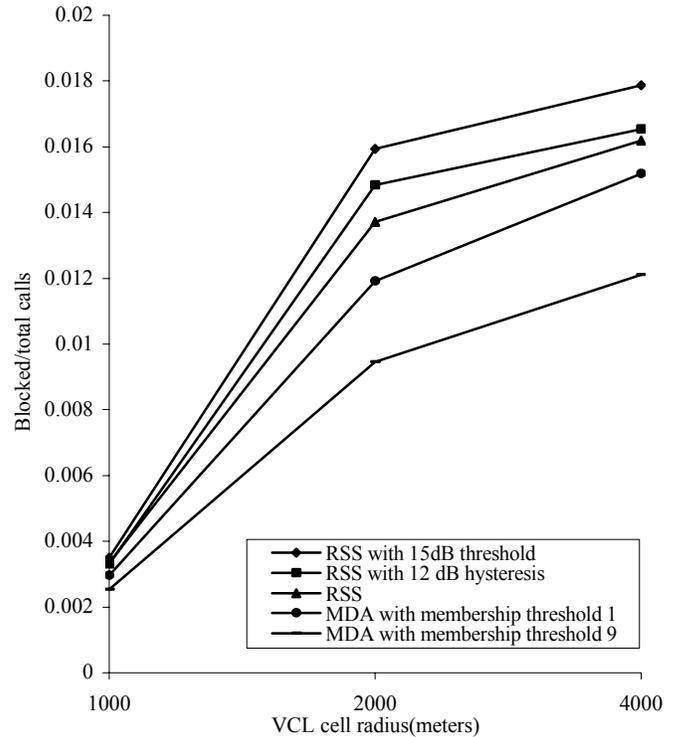
Figure 12. Comparison of handoff decision algorithms for the second scenario, in terms of blocked calls due to lack of network resources for the multiplication factor 1.
