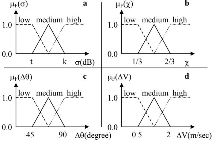
Figure 5. Membership functions of three fuzzy sets, namely, 'LOW', 'MEDIUM', and 'HIGH': (a) for the received signal strength  $\sigma$  (b) for the capacity utilization  $\chi$  (c) for the difference in movement direction  $\Delta\theta$  (d) for the difference in speed  $\Delta V$ .
